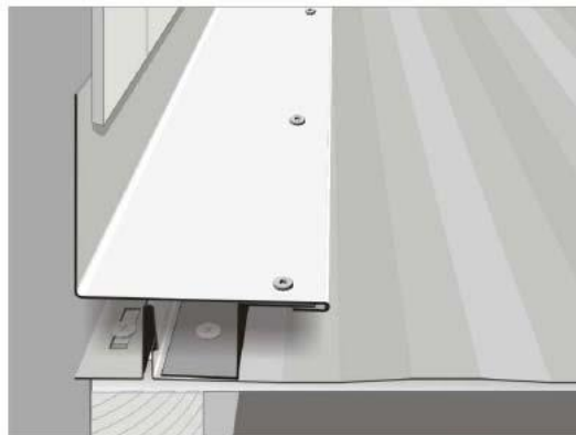
Fig. 17 Standard Sidewall attaches to z-flashing with screws
